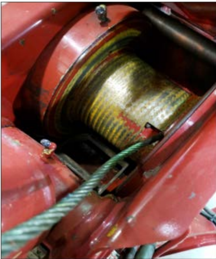
(Fig. 1): Rotate the Wire Rope Drum, until the narrow end of the Wire Rope Socket Wedge is visible
