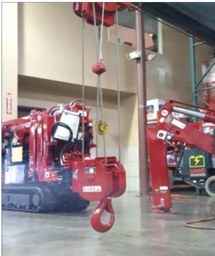
(Fig. 1): WINCH DOWN to lower the hook to the ground, but DO NOT ground the hook via WINCH DOWN.
