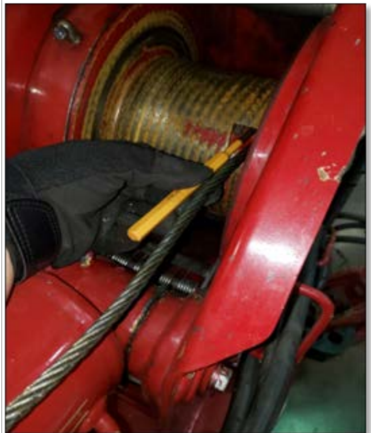
(Fig. 2): Push the Wire Rope Socket Wedge out of the Wire Rope Drum and retain for future use.
