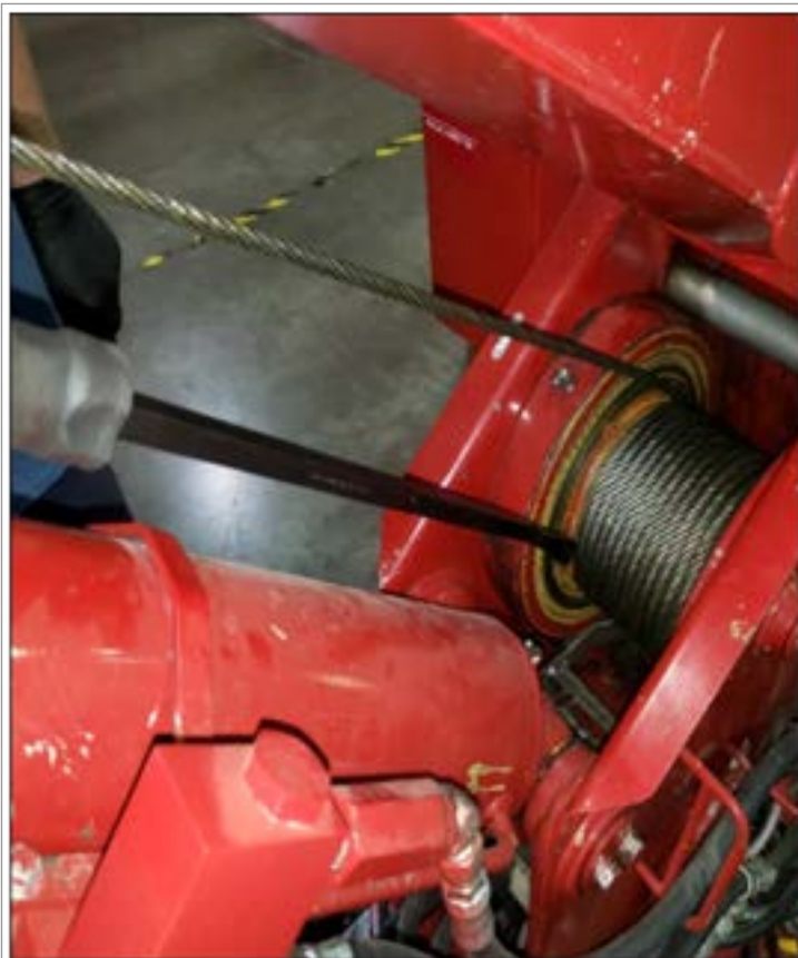
(Fig. 1): Periodically stop WINCHING UP to make that the wire Rope is laying back onto the drum in an orderly fashion.
