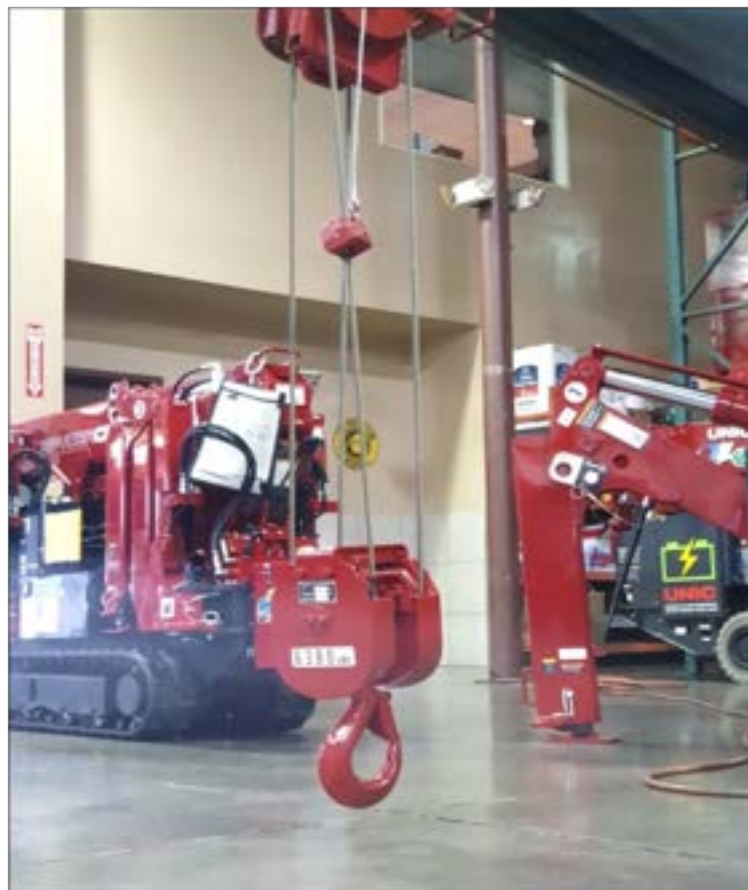
(Fig. 2): Once the hook block is off the ground and there is pressure on the wire rope, you may WINCH UP the hook block.
