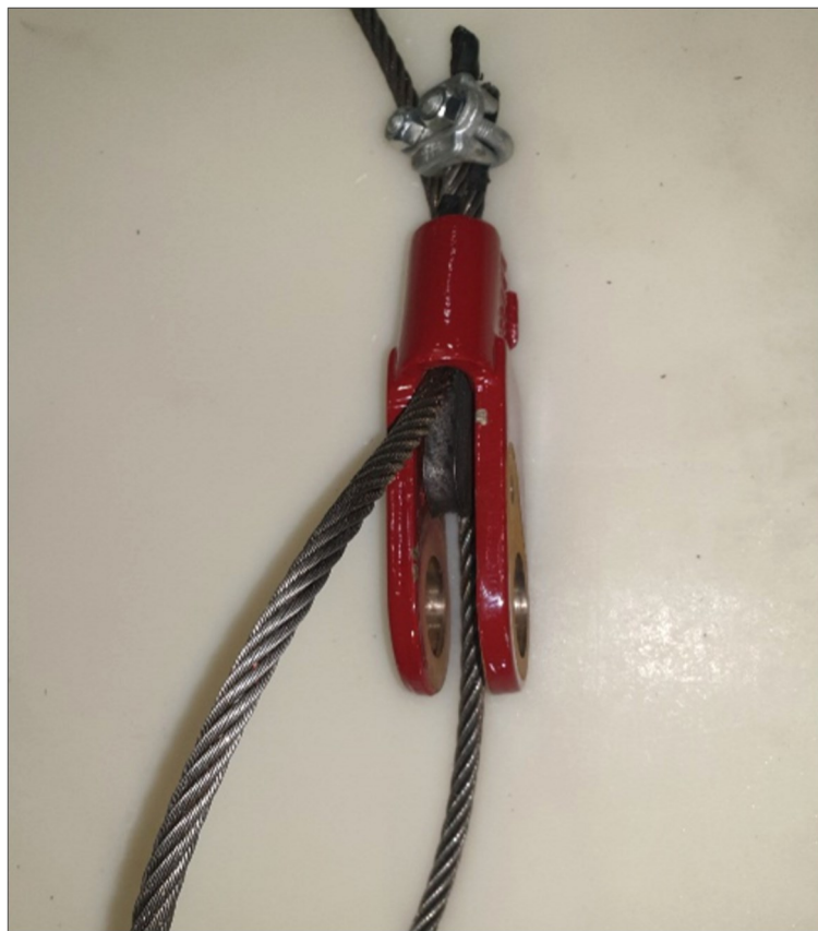
(Fig. 3): When assembling the wire rope clip, make sure to place the U-bolt on the actual wire rope and the saddle on the Wire Rope Spacer.
