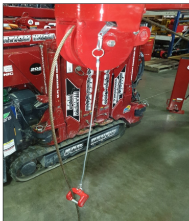
(Fig. 5) The wire rope passes over the right-hand Boom Tip Sheave and Jib Sheave, and through the Jib A2B Weight.
