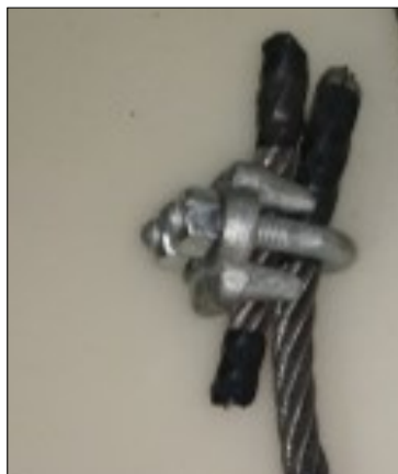
(Fig. 7) The saddle of the Wire Rope Clip sits on the Spacer while the U-Bolt sits on the end of the wire rope.
