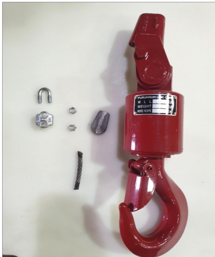
(Fig. 2): Retain all of the parts from the 1-Part Hook Block, including the Wire Rope Spacer
