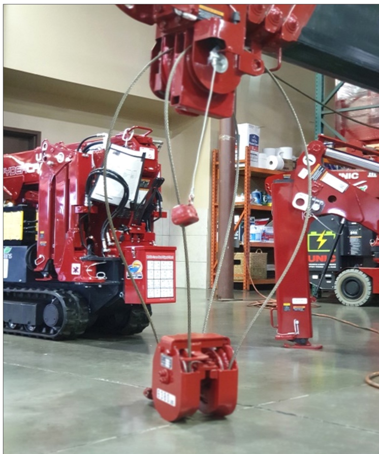
(Fig. 2): BOOM DOWN to actually place the hook block on the ground.
