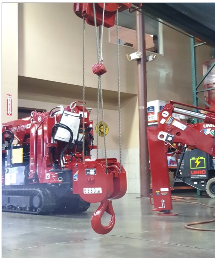
(Fig. 2): Once the hook block is off the ground and there is pressure on the wire rope, you may WINCH UP the hook block.
