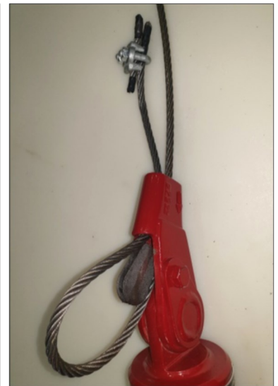
(Fig. 4): Before closing the loop and seating the wedge, make sure you have AT LEAST 6" of end "tail" ABOVE the becket.
