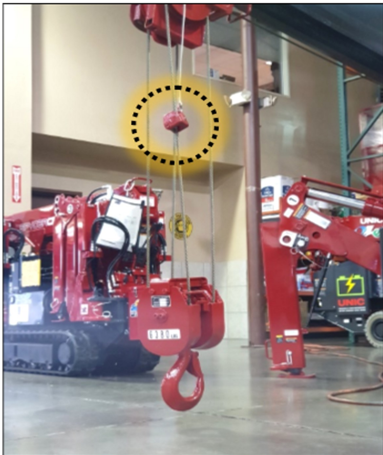
(Fig. 1): You DO NOT need to WINCH DOWN quite this low; once the A2B Weight is pulling closed the A2B Switch, the hook is deployed.
