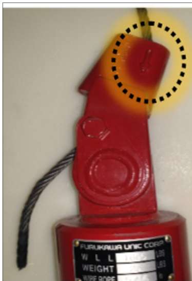
(Fig. 2): Push the end through the top of the becket of the Wire Rope Socket of the 1-Part Hook Block (follow the arrow).
