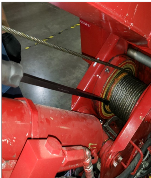
(Fig. 1): Periodically stop WINCHING UP to make that the wire Rope is laying back onto the drum in an orderly fashion.
