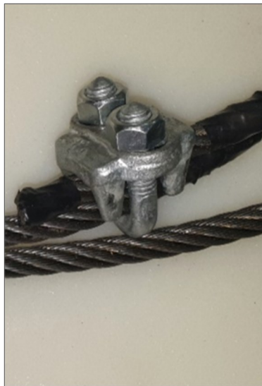
(Fig. 3): When assembling the wire rope clip, make sure to place the U-bolt on the actual wire rope and the saddle on the 8mm spacer.
