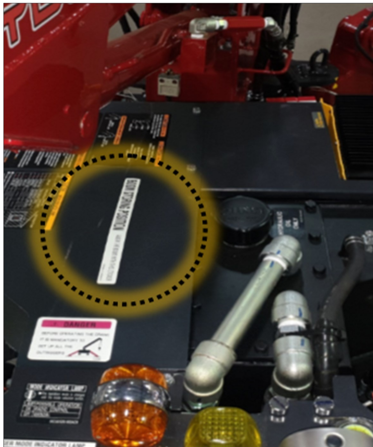
(Fig. 2): The URW094 DOES NOT have a Boom Stored Switch, simply line up the boom with the Boom Stored Decal
