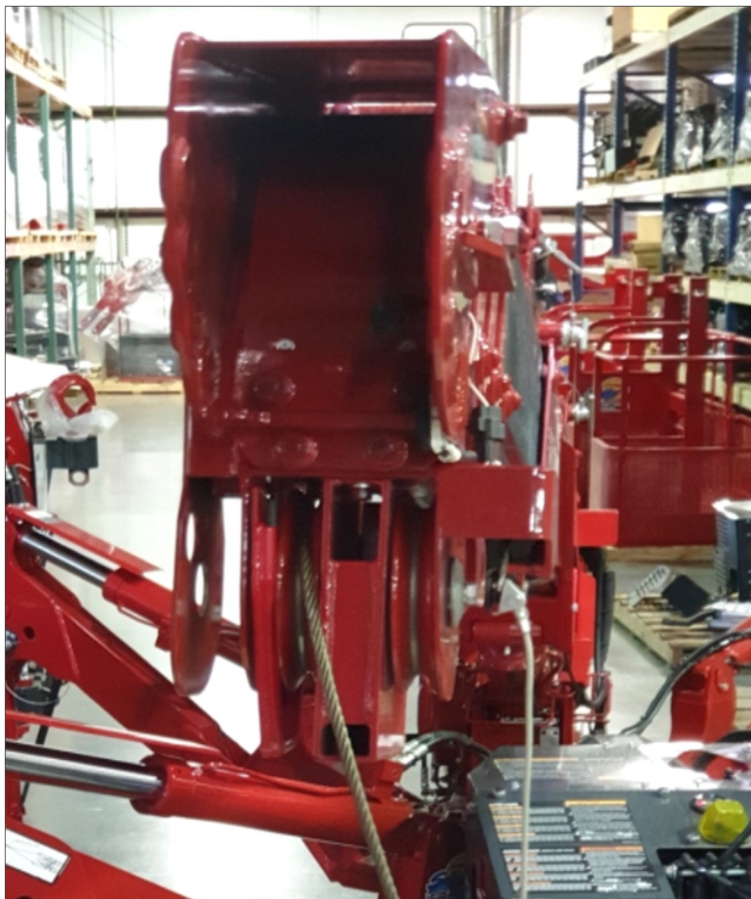
(Fig. 1): Maneuver the boom until it is to the LEFT of the Boom Stored Safety and the Boom Stored Decal on the top of the carrier.
