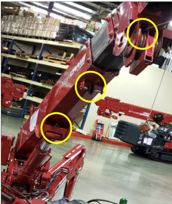
(Fig. 3): Reeve the wire rope through the boom BACKWARDS, starting at the right-hand sheave of the Boom Tip.
