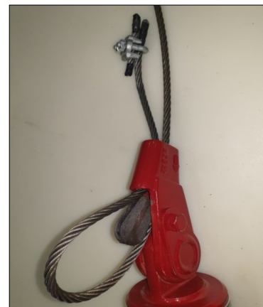
(Fig. 8) Insert the narrow end of the Wire Rope Wedge into the wide side of the becket of the Wire Rope Socket.
