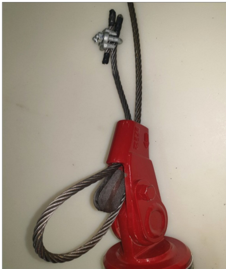
Fig. 1) The 1-Part Hook Block with the Wire Rope Socket Wedge exposed
