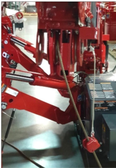
(Fig. 1): The end passes over the right-hand Boom Tip Sheave and through the A2B Weight on its way to the 1-Part Hook Block.
