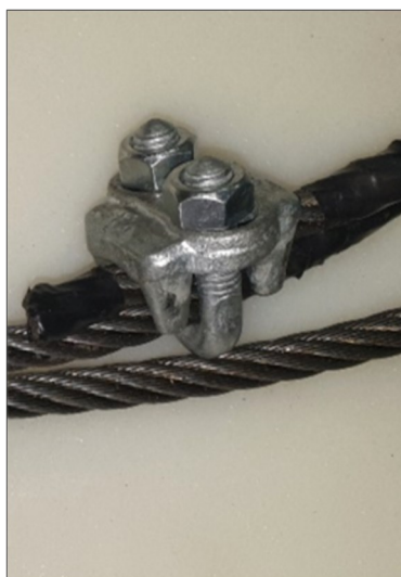
(Fig. 3): When assembling the wire rope clip, make sure to place the U-bolt on the actual wire rope and the saddle on the 8mm spacer.
