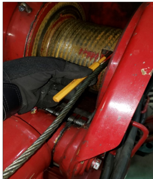
(Fig. 2): Push the Wire Rope Wedge out of the Wire Rope Drum and retain for future use.
