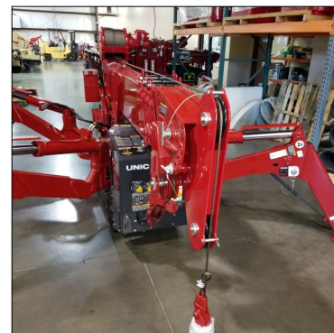
(Fig. 4): The Auxiliary Winch with its wire rope reeved and connected to the 1-Part Hook Block.
