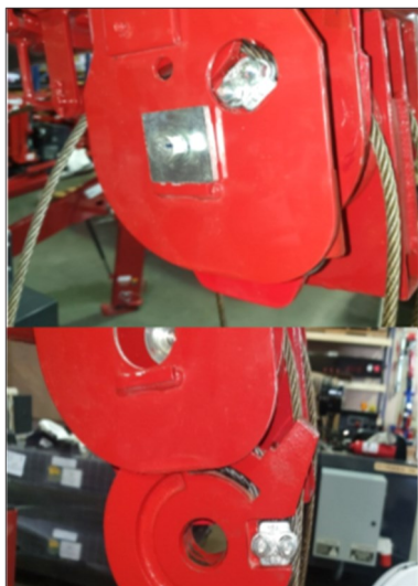
(Fig. 1): Remove the Wire Socket Pin Bolt and then support the Wire Rope Socket as you pull the Wire Rope Socket Pin out.
