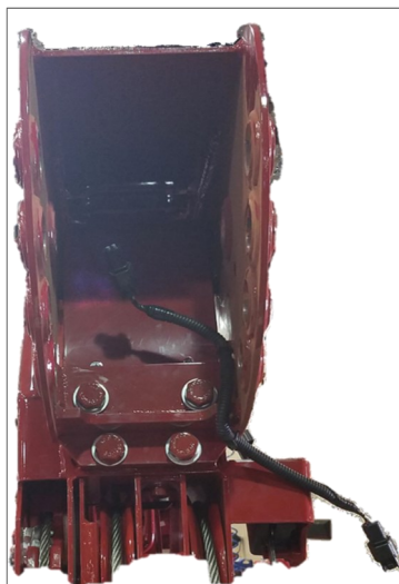
(Fig. 3) The A2B Switch Extension Cord is installed on the inside of the Jib Hood.
