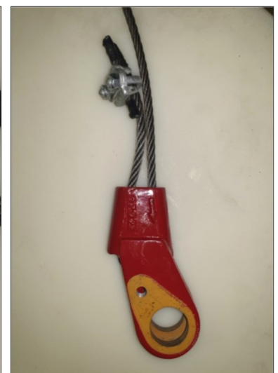
(Fig. 4.): Before closing the loop and seating the wedge, make sure you have AT LEAST 6" of end "tail" ABOVE the becket.
